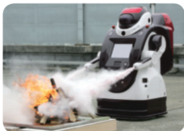
Guard ROBO D1 Type putting out a fire
